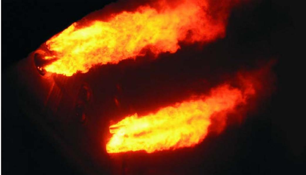
Pulverized solid fuel in a power plant boiler
